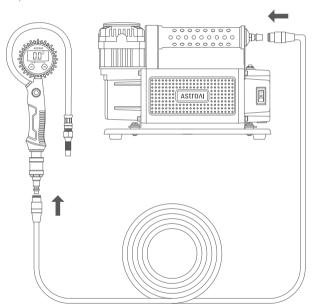
2. Remove the valve stem cap from the tire stem, then connect the airflow controller's quick connector to the valve stem.
