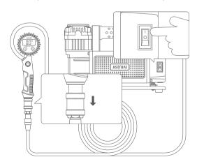
6. Push the airflow valve upwards to stop the air inflow into the pressure gauge. Doing this reduces airflow pressure errors and helps accurately measure the interior pressure value. After getting the pressure value, pull the airflow valve downwards to continue inflating (if needed).
