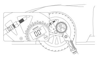
3. Press the LCD Button to turn on the screen. Press it again to choose the desired unit. 4 options: PSI, Bar, kPa, kg/cm².
