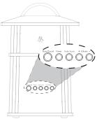
1. Press the Power button on the back of the speaker to turn it on. The indicator light on the front of the speaker blinks while the speaker is tuning to the transmitter. The indicator light turns solid blue when the speaker is tuned to the transmitter-you should hear sound coming from the speaker now.
