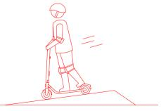
Watch your speed when traveling downhill. Use both brakes together when traveling at high speed.
