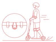
4. Slow down by releasing the throttle. Squeeze the electronic brake and stamp the fender with foot at the same time for a sudden brake.
