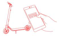
Power on the KickScooter. A blinking Bluetooth icon indicates the KickScooter is waiting for a connection.
