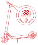
1. Power on the scooter and check the power level. Charge the scooter if the battery level is low.
