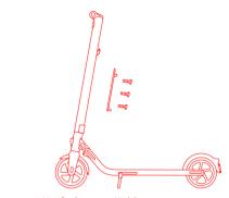
Install the external battery on the rail and fix it with the M4 (20mA). Verify that your KickScooter powers on and off. screws (2 pcs) and M3 screw (1 pcs), provided with this product. After they are properly installed, block the screw holes with the rubber stopper.
