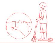
3. Put your other foot on the foot deck to keep both feet stable. Press the throttle on right hand to speed up when you are balanced.
