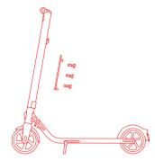
3. Install the external battery on the rail and fix it with the M4 (20mm)Verify that your KickScooter powers on and off. screws (2 pcs) and M3 screw (1 pcs), provided with this product.
