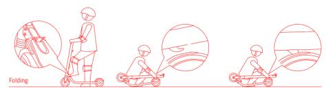
Step on the folding pedal while pushing the handlebar forward slightly. Then fold the handlebar down until it locks into the rear fender.
