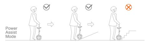
Pull up the guide bar to enter Power Assist Mode (powered on, with no rider). Steer the miniPRO across smooth surfaces using the guide bar. Do not guide it up stairs, across potholes, over large cracked/uneven surfaces, or over other obstacles; guide your miniPRO around the obstacle or carry it over the obstacle as shown in the previous section.
