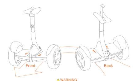
Always step on/off from the back of the miniPRO. Otherwise you risk falls and/or collisions because the steering direction is reversed.
