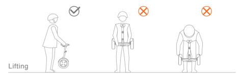
For your safety, motor power is cut off when the miniPRO is lifted off the ground in Balance Mode. When the miniPRO is put back down it will begin balancing again. Do not lift the miniPRO by the fenders or mainframe; you risk pinching or injuring your fingers/hands. Please lift via the steering bar as shown above.
