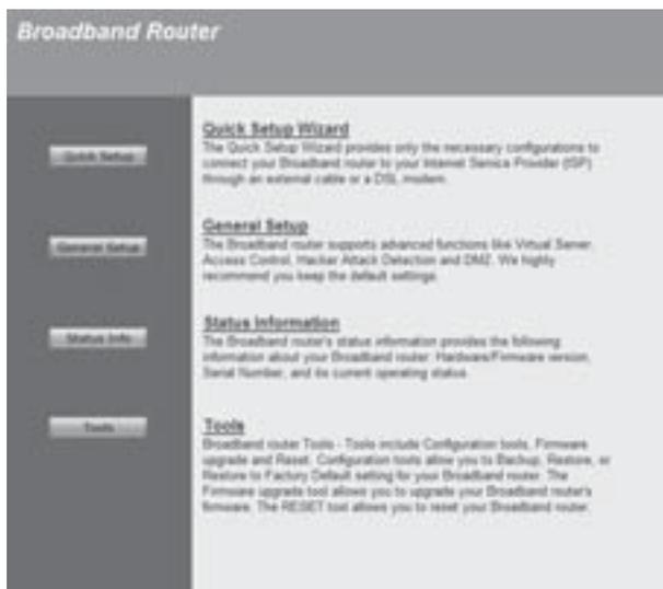
Figure 4 – Router configuration utility
