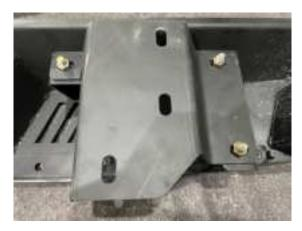
Step 7: It is recommended to install the bumper with assistance. Lift the bumper, align it with the original vehicle mounting holes, and secure it using M12\*35 screws with washers and nuts. Adjust the gap from the vehicle and tighten the screws.
