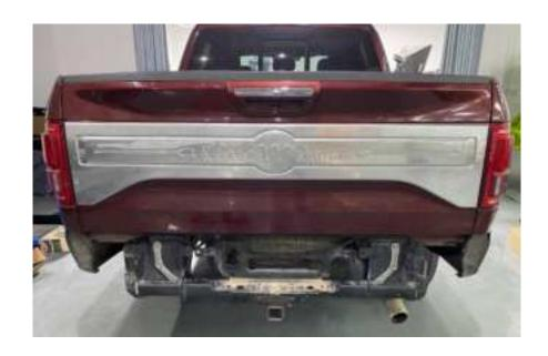
Step 4: It is recommended to install the bumper with assistance. Lift the bumper, align it with the original vehicle mounting holes, and secure it using M12\*35 screws with washers and nuts. Adjust the gap from the vehicle and
