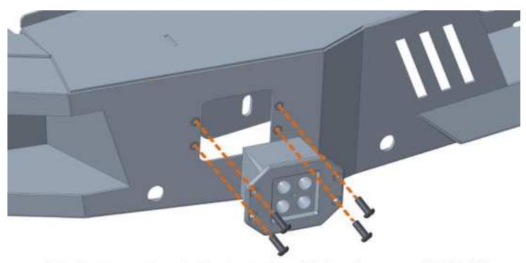
(4) Button Head Socket Cap Bolts Screws (M6\*16)
