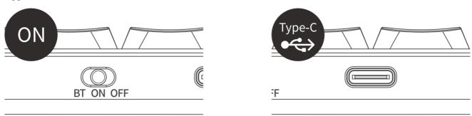
2. Connect the keyboard to the device with attached Type C cable to complete the wired connection mode
