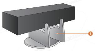
STEP 2. Install the rubber spring( 1) of the Rubber kit list) to the upper mounting bracket( 3) of the Rubber kit list) with washers and lock nuts.
