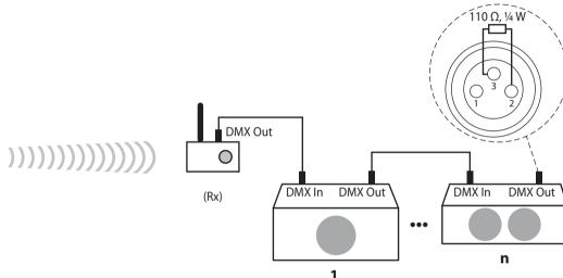
Connect a compatible transmitter to the DMX output of your DMX controller and a receiver to the DMX input of the first DMX device in the DMX chain that is to be controlled. In this point-
