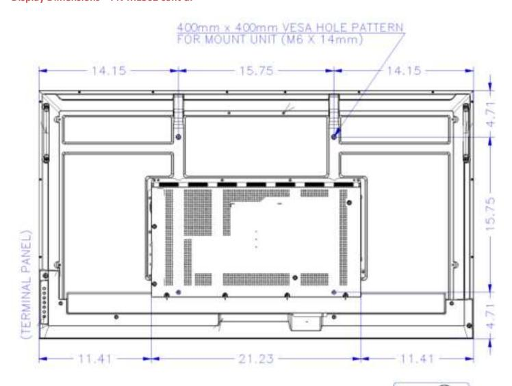
NEC strongly recommends using size M6 screws (14mm + the thickness of the bracket and washers in length).
