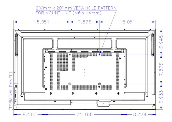
NEC strongly recommends using size M6 screws (14mm + the thickness of the bracket and washers in length).
