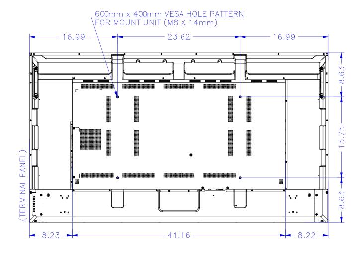
NEC strongly recommends using size M8 screws (14mm + the thickness of the bracket and washers in length).
