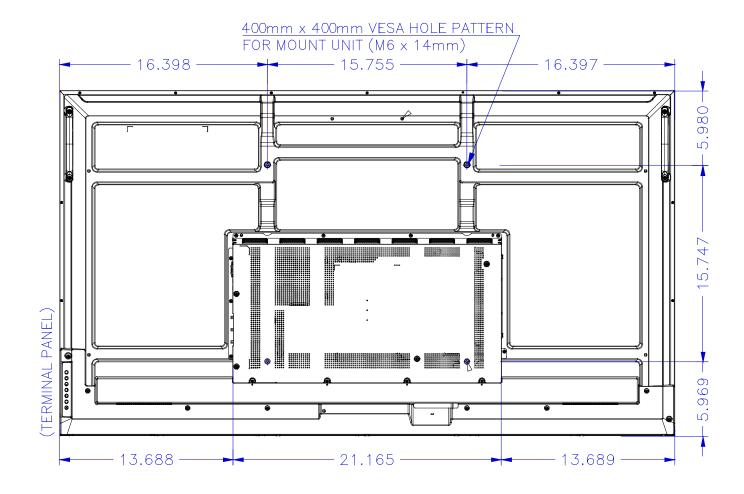
NEC strongly recommends using size M6 screws (14mm + the thickness of the bracket and washers in length).
